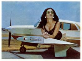
LAMINAR FLOW WING... This is a low-drag, high performance wing. All metal, wrap-around wing skins are flush-riveted and control surfaces are gap-sealed to minimize drag. The Mooney wing affords maximum strength and performance.
