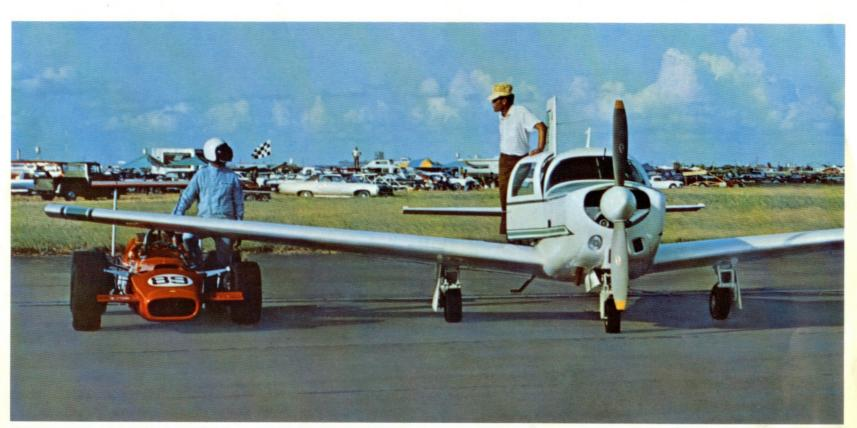
ELECTRIC GEAR — WIDETRACK STABILITY . . . Electrically operated retractable landing gear is standard equipment on all Mooney aircraft except the CADET. The Mooney retractable gear system is the fastest flying — 3 seconds up and 2 seconds down! Wide stance, tricycle gear and steerable nose wheel make ground handling easy. Crosswind and high wind conditions are no problem with Mooney's widetrack stability and shock-absorbing gear.
