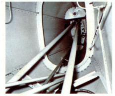
PUSH/PULL CONTROL RODS instead of wire lines and pulleys provide safer and more positive aileron and rudder control and instant response. This feature is the most positive method of connecting the pilot to the control surfaces.
