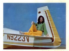
FULL TRIM TAIL · . . Pioneered and perfected by Mooney. The entire horizontal and vertical tail section trims as a unit for best angle of attack and maximum performance.
