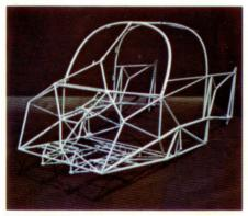
ROLL BAR CABIN ... for an extra measure of safety. Unique among today's competitive models, Mooney adds the security of an all-steel, energy-absorbing, tubular structure completely surrounding the passenger area.
