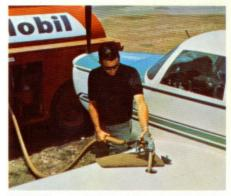
FUELING . . jet-type integral wing tanks are easy to fill. Each fuel cell has a sump drain located under the wing for easy sampling. The sealed, wet-wing tank is easy to maintain and is an added safety feature.
